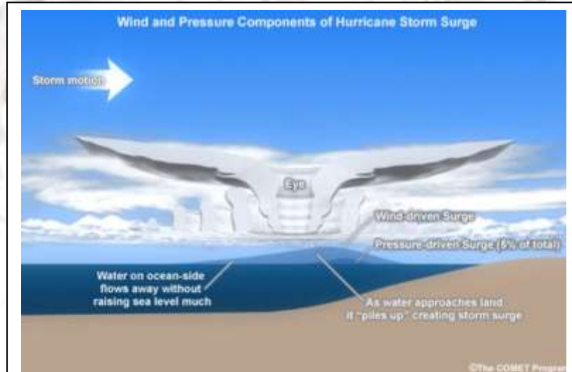
Fig. 5. A Storm Surge is a rise in water level on the land side of a cyclone eye. As the cyclone approaches land, the storm surge gets higher. Higher water level at high tide increases the effect of the storm surge in coastal areas
